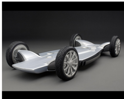
The 2000 GM AUTOnomy skateboard chassis concept (image credit: General Motors)
