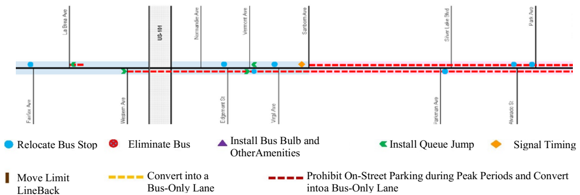
Example of Mix of Types of Bus Priority Treatments (for illustrative purposes)
