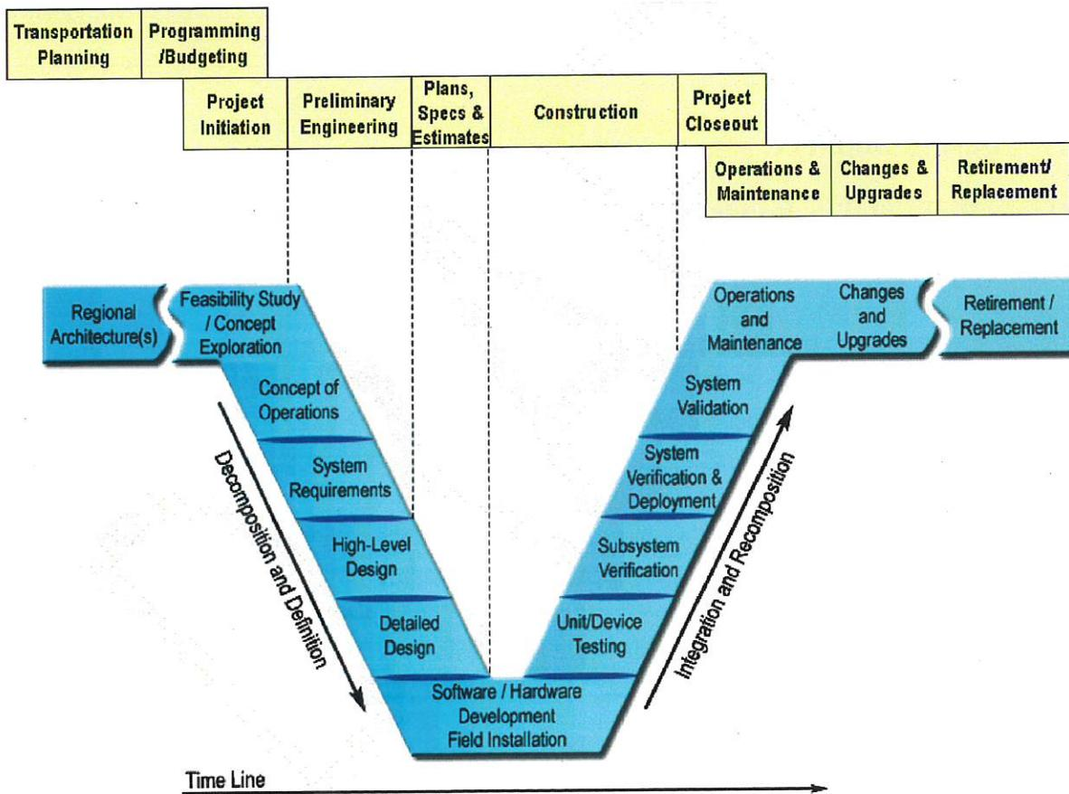
**Figure 2: System Engineering Process**
