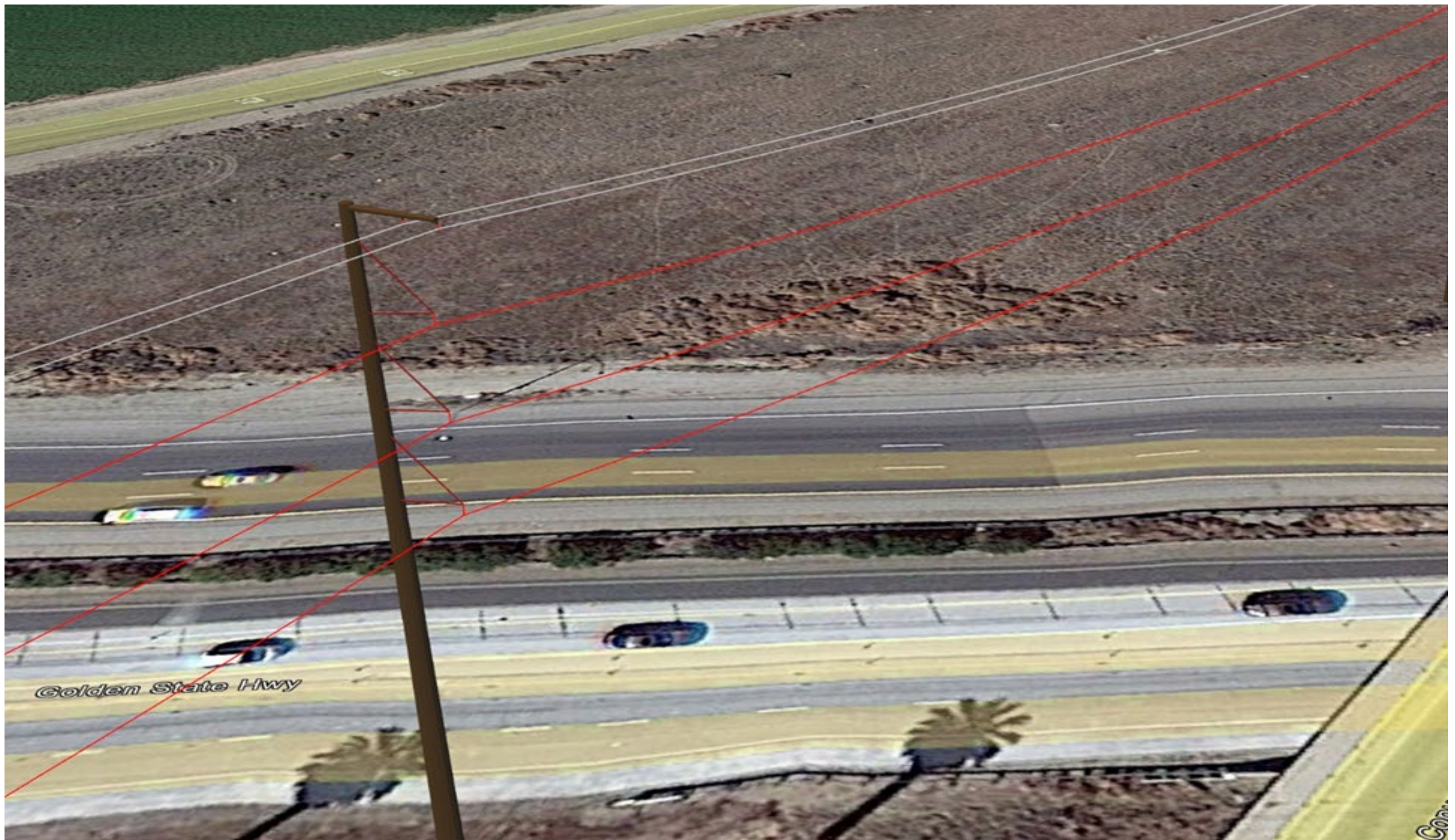
Computer rendering of proposed project – two upper lines (white) are fiber optic lines, three separated electrical lines (red)
