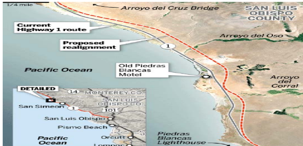
3-mile Realignment to protect HWY from erosion
